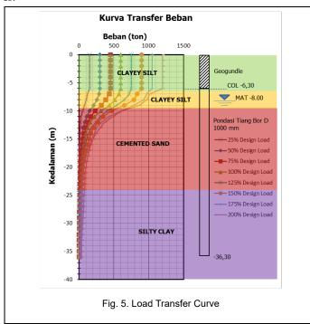
Based on the Load Transfer Curve, the t-z curve can be obtained which is the skin friction of the pile  $(\tau)$  and the displacement due to the movement of the pile (z) and also the q-z curve which is the relationship curve between the end of the pile (q) and the displacement at the pile bottom (z). Figure 9 and Figure 10 shows the t-z and q-z curves.
