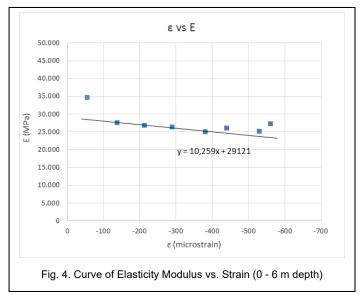
From the curve of modulus elasticity of the concrete vs strain above, the relationship is obtained in the line equation y = 10.26x + 29121. This line equation will be used to determine the elasticity modulus along the pile based on the strain measurement from the fiber optic sensor readings.
