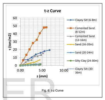
From the t-z curve it can be seen that the skin friction resistance that is mobilized is only up to a depth of 20 m, in other words at depth more than 20 are still in elastic condition. The friction resistance value in the cemented sand layer can reach 48 tons/m<sup>2</sup> meaning that most of the load is carried by the layer.
